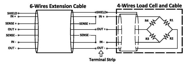
Color and signal matching for a 4-wires load cell:
