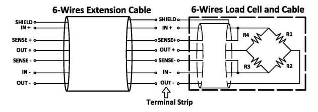
Color and signal matching for a 6-wires load cell:
