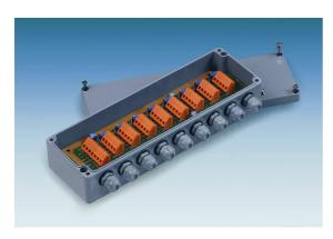
The Junction Boxes are used to connect a group of load cells of the same scale to an electronic indicator, in order to obtain the summing signal of each load cell. The inner precision potentiometer allows a fine tuning for equalizing the weight reading obtained from each supporting point (corner adjustment), when same load is applied on each corner.
