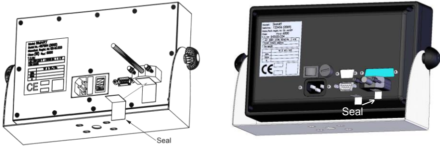
Figure 5.1.1.1 Load cell connector sealing
