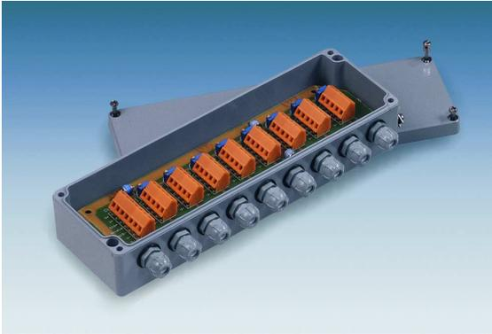
The Junction Boxes are used to connect a group of load cells of the same scale to an electronic indicator, in order to obtain the summing signal of each load cell. The inner precision potentiometer allows a fine tuning for equalizing the weight reading obtained from each supporting point (corner adjustment), when same load is applied on each corner.
